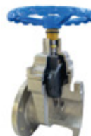
SERIES 200D RESILIENT SEAT GATE VALVE NP16 NON-RISING STEM FLANGED END Material construction in CF8M Vulcanize wedge EPDM WRAS Epoxy paint FBE Min 250 Mic WRAS Working pressure 1.0Mpa 1.6Mpa
