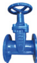
SERIES 200D RESILIENT SEAT GATE VALVE BS5163 NON-RISING STEM FLANGED END DIN pn10/16 Made of Ductile Iron GJ5500. Vulcanize wedge EPDM WRAS Epoxy paint FBE Min 250 Mic WRAS Face to face EN 558 Serie BS5163
