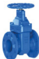
SERIES 200D METAL SEAT GATE VALVE NP16 NON-RISING STEM FLANGED END Made of Ductile Iron GJ5500. Vulcanize wedge EPDM Epoxy paint FBE Min 250 Mic Working pressure 1.0Mpa 1.6Mpa Flanged ends DIN NP 10/16
