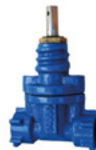
SERIES 210A RESILIENT SEAT GATE VALVE NP16 THREADED END Made of Ductile Iron GJ5500. Vulcanize wedge EPDM WRAS Epoxy paint FBE Min 250 Mic WRAS Working pressure 1.0Mpa 1.6Mpa Threaded ends DIN 259 ( GAS/NPT )
