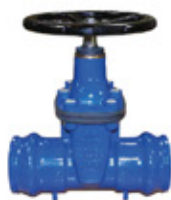
SERIES 220D RESILIENT SEAT GATE VALVE NP16 NON-RISING STEM PVC END Made of Ductile Iron GJ5500. Vulcanize wedge EPDM Epoxy paint FBE Min 250 Mic WRAS Working pressure 1.0Mpa 1.6Mpa
