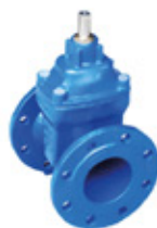
SERIES 200D RESILIENT SEAT GATE VALVE NP16 NON-RISING STEM FLANGED END S Made of Ductile Iron GJ5500. Vulcanize wedge EPDM con WRAS Epoxy paint FBE Min 250 Mic con WRAS Working pressure 1.0Mpa 1.6Mpa
