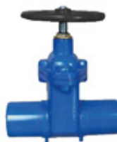
SERIES 210A RESILIENT SEAT GATE VALVE NP16 VERTICAL THREADED END Made of Ductile Iron GJ5500. Vulcanize wedge EPDM WRAS Epoxy paint FBE Min 250 Mic Working pressure 1.0Mpa 1.6Mpa Threaded ends DIN 259 ( GAS/NPT )
